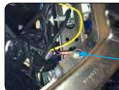
5. Connect the Power Module to Power Cable.
