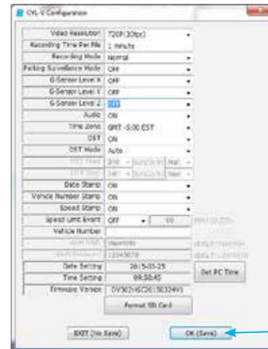
CYL-V Recorder is supplied with a factory default configuration, see below for specific default settings. If the factory default settings are acceptable, there is no need to do anything further. Simply insert the Micro SD card into the Recorder, and begin driving.
