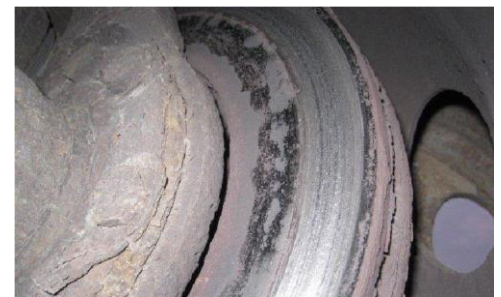
Metal-to-metal contact. OOSC, Part II, a.(6)(c) / 393.48(a)-U.S.
