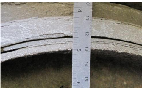
Worn out linings. OOSC, Part II, a.(5)(c)vii / 393.47(d)(2)-U.S.
