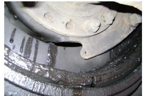
Contaminated lining. OOSC, Part II, a.(5)(c)vi / 393.47(a)-U.S.
