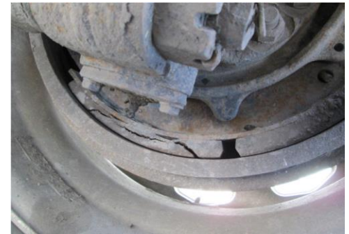
Cracked lining. OOSC, Part II, a.(5)(c)iii / 393.47(a)-U.S.
